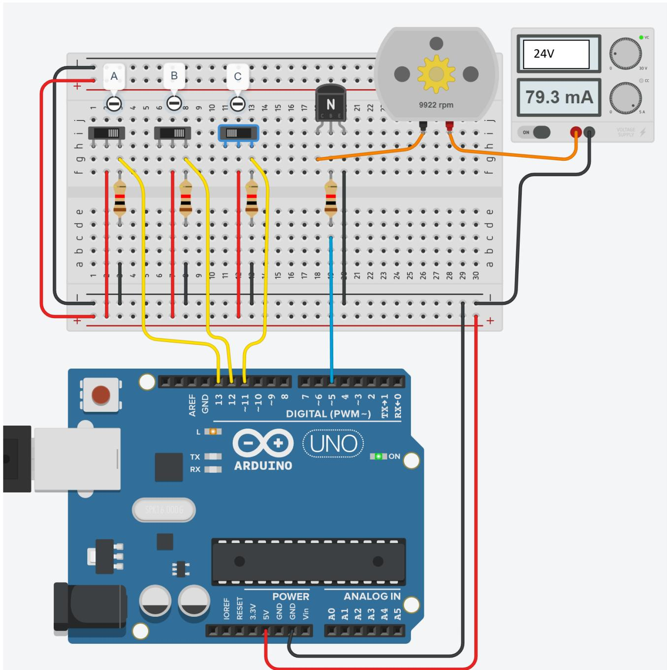
$$I_c = 10W / 24V \text{ (A)} \rightarrow I_b = I_c / h_{FE} \text{ (A)} \rightarrow R_b = (5V - V_{be}) / I_b \text{ (ohm)}$$
